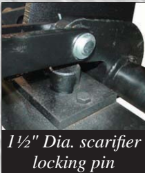
Cylinder raises scarifier beam
