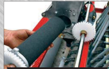
Easy Disassembly of Rollers
