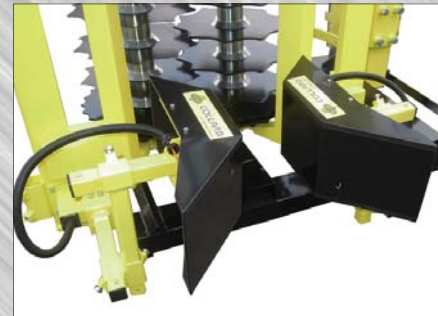
Magnetic sensors - Open and close cutting heads when sensing steel posts
