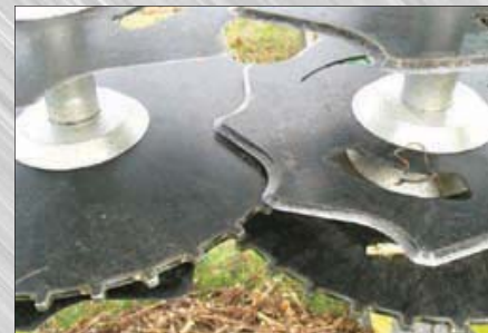
Cutting blades and notched discs for clean cuts and trellis post protection
