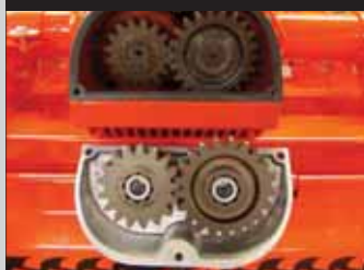
Quick change speeds on 4 Speed Gearbox
