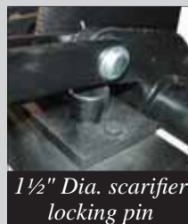
Cylinder raises scarifier beam
