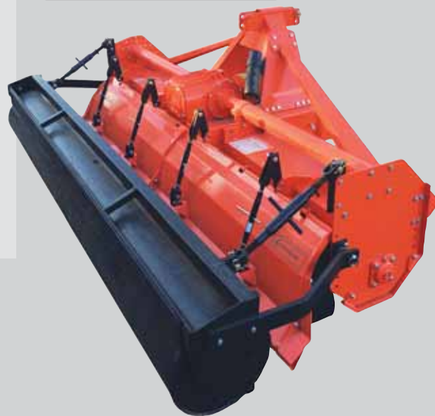
O.E.M. Tines Tillers Feature Bonded Tungsten Coated Tines
