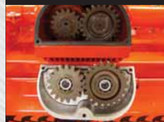
Quick change speeds on 4 Speed Gearbox
