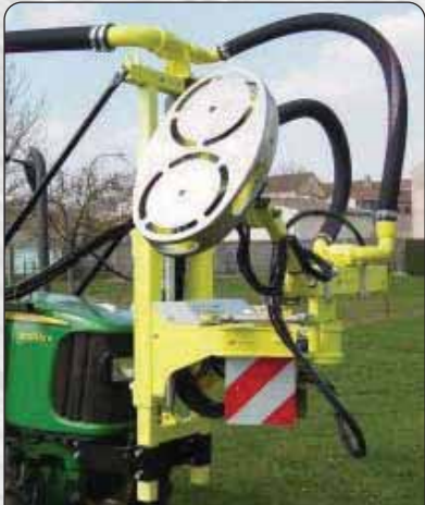
Elliptical shaped dual rotor defoliation head
