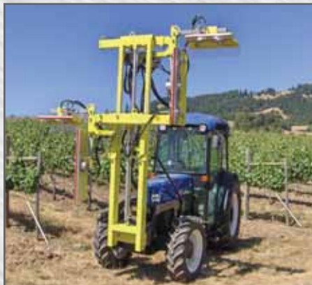
Model P2200TS Trims 2 Half Rows, Terraced Vineyard
