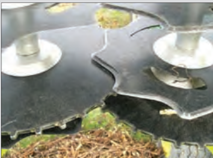
Cutting blades and notched discs for clean cuts and trellis post protection
