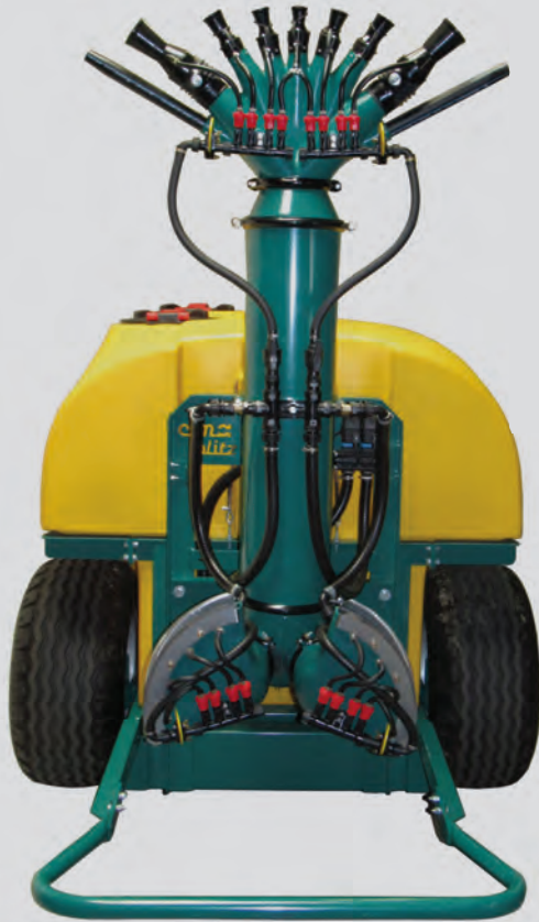
Hops distribution head with 7 upper cannons and 2 large lower fishtail nozzles with 128 spray outlets.
