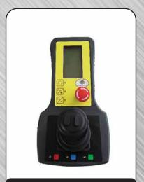
Joystick for control, adjustment and safety stop button
