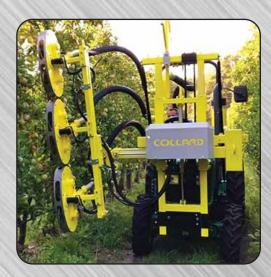
Effective leaf removing to aid in ripening, color intensity and removing any impurities. The leaf removal is achieved by our "patented" double flow low pressure air produced by the 3 point PTO driven air compressor. The Collard system blows through the leaves at fruit level by rotating nozzles that removes the leaves from both the outside and interior of the row, achieving selective leaf removal around the apples without damage.
