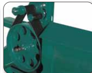
Power band fan speed up system with built-in overrunning clutch
