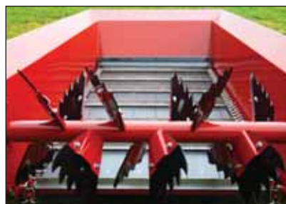
Beater paddles are bolt on for easy replacement
