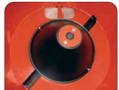
Coned material diverter & full length agitator blades
