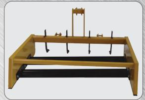
Arena Maintenance - Set the shanks at the maximum depth and lower the dual cutting edges to the maximum depth. This operation will move the material away from fences, and loosen, aerate, and smooth out the surface.
