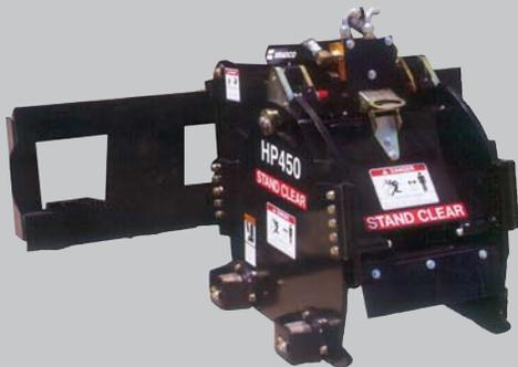
For standard flow and high flow models available for skid-steer loaders. 12" to 40" planing widths available 0" to 5" planing depth. Manual depth and tilt option available on standard flow.
