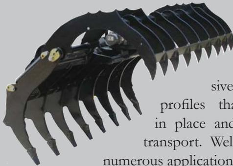
Remove the toil and leave the soil at your job site with aggressive tine and grapple profiles that lock material in place and stabilize during transport. Weld-on D-Ring for numerous applications, replaceable pin-on H&L-230 style teeth for durability, serviceability, & extended life. 72", 78", and 84" widths available; 49" grapple opening. For skid-steer loaders.
