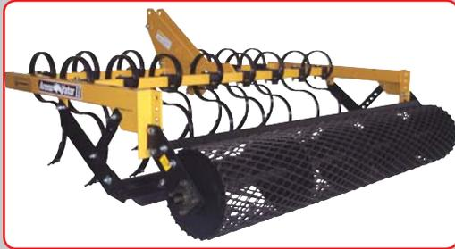
The *AV Series* of Arena-vators were designed to renovate and condition horse arenas and tracks in a single pass. The machines consist of two rows of vibrating S-tines to loosen and cultivate the soil, an adjustable bar to level the soil and a rear roller to help gauge the depth. The rear roller is available with mesh or spiral rod, depending on the finish you desire.
