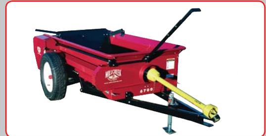
The *57 Series* spreaders is recommended for up to 10 horse stables and is available in ground wheel or tractor PTO drive. The poly floor is standard and guaranteed for 20 years. The spreader operates efficiently, pulled by a tractor 18 horsepower and above.
