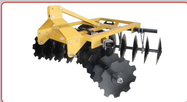
Our *T Series* of tandem discs are an economical way for tilling pastures. The discs have two rows of blades; cutting notched blades on the front gang and finishing smooth blades on the rear gang. The discs are available with 18 inch diameter blades, with widths of 60", 72" and 84". These discs will level and mix the soil. Any of your arena tools (see arena maintenance) can then finish the soil for seeding.
