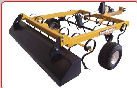
The *Arena-Vator Junior* is a complete self contained towable implement that can be operated by almost any vehicle. The tilling depth is controlled by an electro cylinder operated from the vehicle seat. The unit is also available with a manually operated turnbuckle. The two rows of "S" tine shanks vibrate in a circular motion when contacting the ground, thus loosening and cultivating a large area around the shank points. The adjustable rear finishing box contains and levels out the soil.
