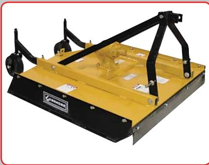
Our *Model L-48-40-XB* Rotary Mower was developed for tractors 15 to 20 horsepower. Stability is very important for small tractors, especially in mowing rough terrain. Two rubber gauge wheels keep the mower level, and takes stress off the tractor by giving the mower a more stable footprint. This mower has an overall width of 51 inches.
