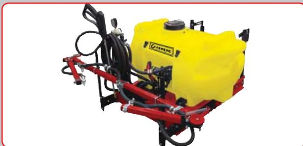
Our *Model UTL-40-5* sprayer with 40 gallon poly tank will handle most spraying projects around the ranch. The simple electric pump is powered by the battery on your towing vehicle. This diaphragm pump was designed to handle herbicides. Standard equipment includes handgun with 25 feet of hose and boom with 100" coverage.
