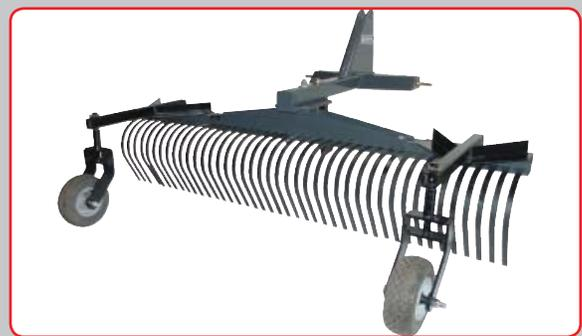
Our **LR Series** of rakes are a great tool for building and maintaining roads. The rakes can be set in the angle position to remove stones and debris. Then gravel can be distributed evenly over the base material. As time passes, you can then re-level over the entire roadway. These low cost implements are available in 5, 6, 7, & 8 foot widths. The gauge wheels are an option.
