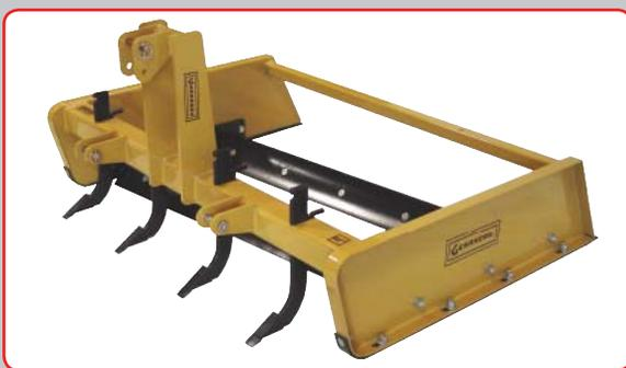
Our **Grading Scrapers** are an excellent implement for access road maintenance. The dual blade, flow through action cuts out high spots, fills holes, and moves material from the outer edge of the road toward the center, thus achieving a smooth finished road. These compact scrapers are available in 5, 6, & 7 foot. This is an extremely easy tool to operate.
