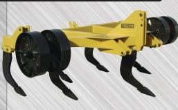
The GE Series of 3-point hitch mounted Rippers was designed for extreme duty subsoiling. The Rippers have A.S.A.E. quick hitches for Cat. 3 and 4N tractors. The shanks are "L" style, 1 ½" thick by 36" long. Optional gauge wheels are available in signle or dual steel wheels and single or dual rubber tires.
