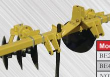
Our Ridgers were built for heavy duty use. The gangs are adjustable for tilt and pitch and are available in 3 or 4 blades. The 3-point is Cat. 2, A.S.A.E. quick hitch. The main beam is 4" x 6" x ¼" wide by 8 foot long. Blades are on 9 inch centers with cast iron spacers.
