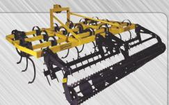
This Gearmore implement combines three different operations in order to obtain the maximum in soil conditioning. First the vibrating "S" tines break up the ground, then the spring loaded spike tooth bar levels and breaks up clods. The final operation is the spring loaded 12" diameter crumbler roller, which mulches and finishes leveling the soil. These Soil Conditioners are ideal for seedbed preparation on most crops.
