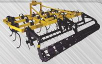
These 3 in 1 soil conditioners combine heavy-duty "S" tines to break the soil. A spring loaded spike tooth bar follows the "S" tines to level the soil and break clods. Then the aggressive spring loaded rolling crumbler completes the work by creating a fine, level surface. This one pass operation leaves orchard rows level, weed free, and manicured to impress your neighbors.
