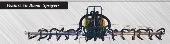
Our Venturi Air Boom Sprayers were developed to obtain total plant coverage, especially the underside of leaves. This system of fine micron droplet spraying achieves the following benefits: spray atomization of droplets are smaller and more uniform, less fill-ups, even distribution of concentrated spray, better product utilization, less chemical waste, and soil/water contamination. These air boom sprayers area available in 23, 27, or 40 feet.
