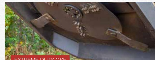
**Intended Use:** The Ground Shark™ Brush Cutter is designed for cutting brush and small trees up to 10" (178mm) in diameter while maintaining a 12" (305mm) maximum ground clearance. When equipped with the tooth kit, the attachment will also grind the remaining stumps down to ground level. Use in any other way is considered contrary to its intended use.
