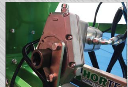
PTO driven dual hydraulic pumps and speed-up gearbox
