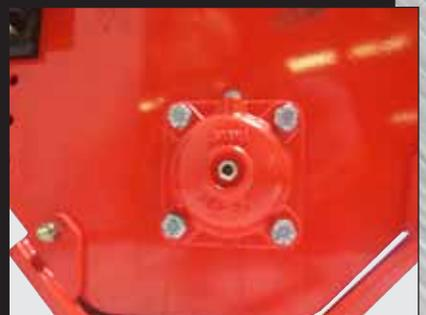
are mounted in heavy cast hubs. This assembly is an oil bath system for cooling the bearings to insure long life.
