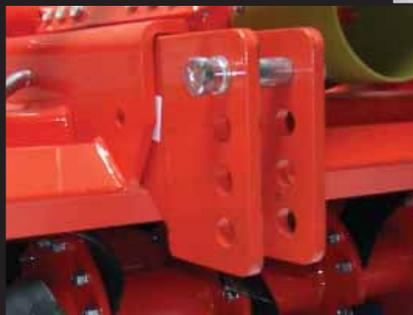
have 4 positioning pin holes. This allows the tillers to be mounted on all tractors no matter what diameter tires.
