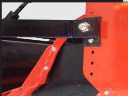
tailboard/hood side mounted soil containment plates to prevent ridges in the soil.
