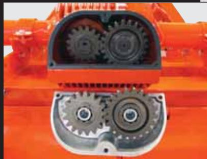
has quick change gears to obtain the best rotor speeds for 540 or 1000 RPM tractors.
