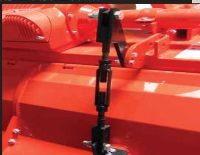
lock the rear tailboard in place so the exact amount of soil is released to the rear roller.
