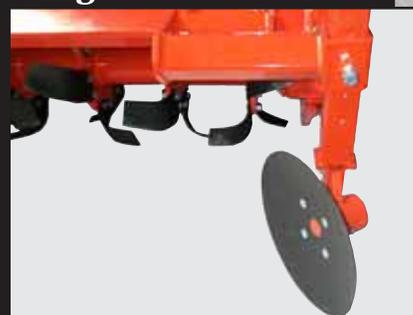
to cut and feed material into the tilling chamber. This eliminates grass build up on the skids and aids in leveling the orchard floor.
