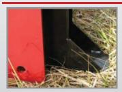
Standard on HPD-16/22Q/26Q SHC. Big-foot stabilizer provides sure footing for driving those larger posts, reducing the driving shock load to the tractor.
