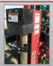
First to install rubber shield around ram driving head, reduces flying wood chips and debris.
