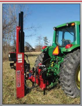
Designed and engineered for those who have serious fencing to do. These center mounted units offer all the quality features of the basic HPD-16 & HPD-22Q plus effortless hydraulic driver alignment controlled by two 3" x 6" hydraulic cylinders. For increased driving force, the heavy duty HPD-26Q SHC delivers 110,000 lbs. of high impact force for driving large posts in tough soil conditions. Big foot stabilizer helps control tractor bounce on these larger units.
